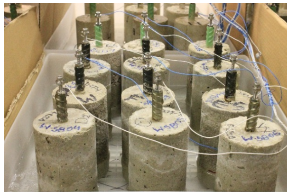
Figure 9: Batch of Specimens Exposed to Mild Water that Includes those Evaluated in this Thesis
