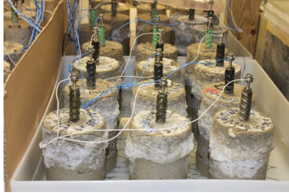
Figure 10: Batch of Specimens Exposed to Salt Water that Includes those Evaluated in this Thesis
